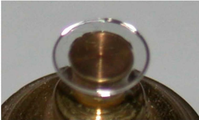
Photograph of 1 mm size WGM resonator disk
