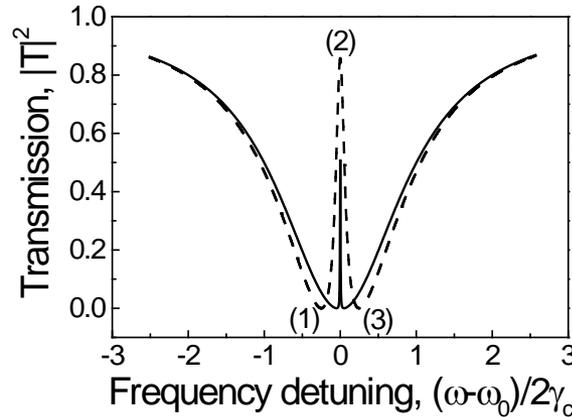
The width of the transparency resonance (2) depends on the resonators' frequencies
