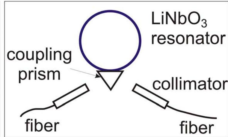
Optical coupling scheme for the disk resonator
