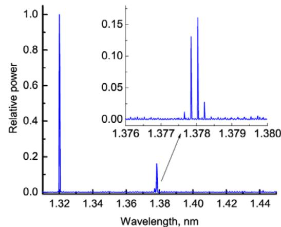
The spectrum of light exiting the Raman-active WGM resonator. The inset shows the structure of the Stokes line. The wavelength difference between the peaks shown in the inset corresponds to the free spectral range of the resonator.
