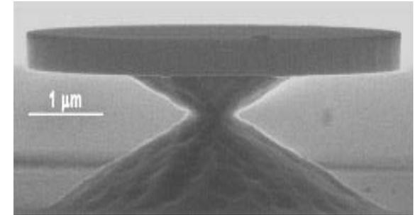
Silicon microdisk,  $Q \sim 5 \times 10^5$
