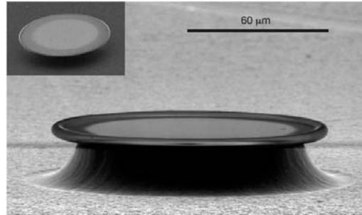
Fused silica microtoroid  $q \sim 1 \times 10^8$
