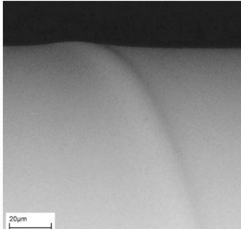
STM picture of a single mode resonator being a “rim” over a multimode waveguide
