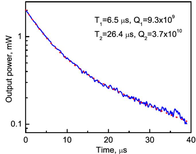
Typical ringdown characteristics of the fluorite WGM resonator. The solid line corresponds to the experimental observation, and the dotted line – to the theoretical simulation.
